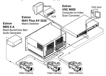
Figure 2-23 — Multiple device external sync connection example
